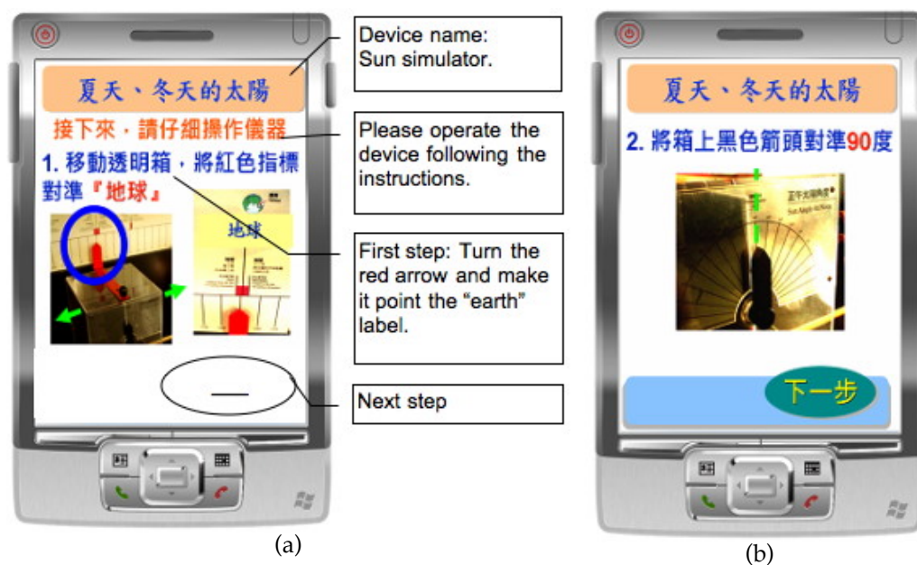
Figure 5: Example of guiding the student to operate the target device
