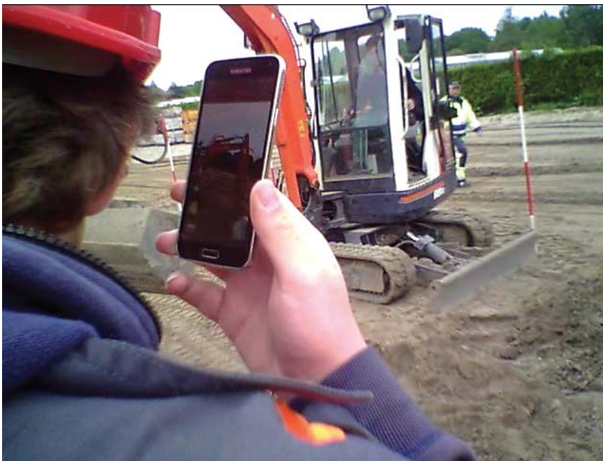
Figure 5. Field case study at BauABC: The cause of noise needs to be determined. The instructor and the group are looking at the joints and pointing to them using the SoAR drawing feature. The instructor asks the group of apprentices whether the procedure of lubricating the joints has been followed.
