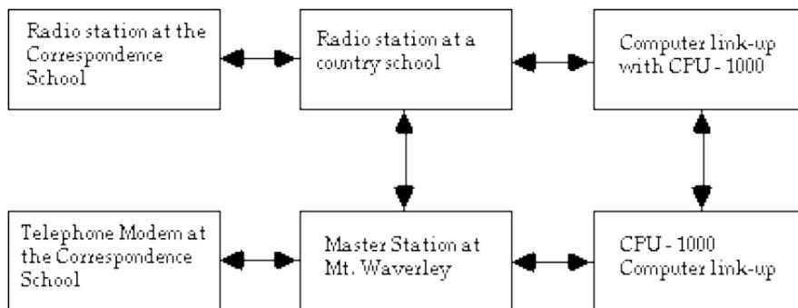
**Figure 1: Radio-Modem set up**
