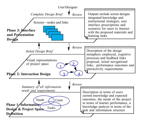
Figure 1: The design process used as the basis for interactive multimedia project development (Hedberg et al, 1994).
