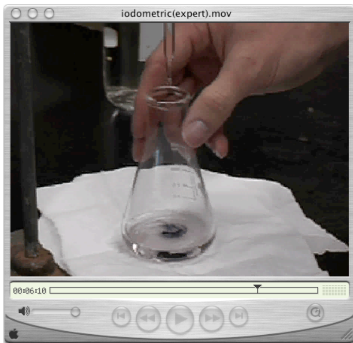
Figure 2: A still image taken from the QuickTime movie illustrating a technical component of the laboratory procedure for measuring preservative levels in wine, showing the colour of the indicator at the end point of the experiment.
